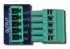
This connector provides 3 digital outputs for control of external devices. Output assignment is controlled in software.
