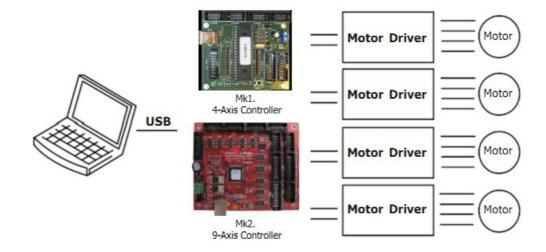
The planet-cnc.com series of USB CNC motion controllers link between a personal computer and motor drivers supporting step/dir control. They are compatible with most drivers. The controllers use the USB port, available on all modern computers and laptops. They can serve as direct replacement or upgrade for many parallel port break-out boards.
