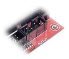
This connector provides 7 digital outputs for control of external devices. The optional 'Output board' links to the Mk2 controller using this connector. Output assignment is controlled in software.
