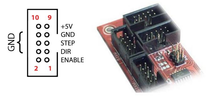
Each connector controls one motor driver.
