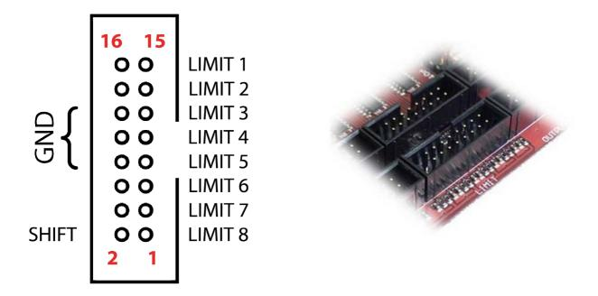
LIMIT 1-8 connects limit switches. It's recommended that a 100nF capacitor is connected directly across switch terminals.
