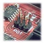
A potentiometer attached to this connector provides a manual jog speed control when using jogging keyboard connected to *JOG* connector.
