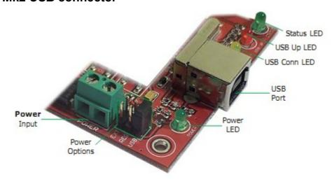
The Mk2 USB CNC controller connects to computers via the USB port. The port uses the USB 2.x standard.
