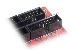
This connector provides inputs for use with axis, distance and E-Stop switches. MPG pendant devices can also be attached.
