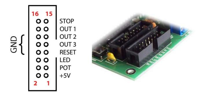
This connector provides for control of external devices and other helpful features built into controller. Pins 2,4,6,8.....16 provide the 'Ground' side of connections.
