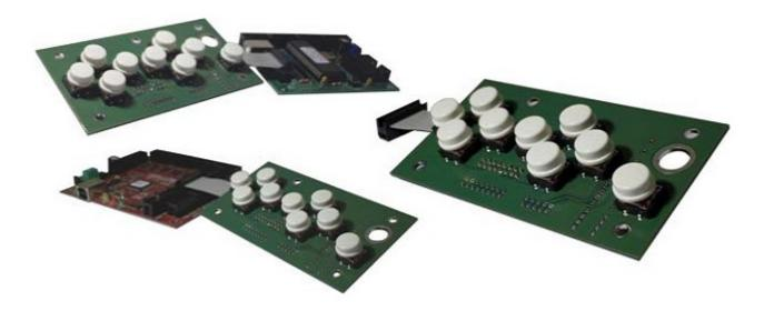
The jogging keyboard is a quick, easy and inexpensive means to add dedicated manual jogging buttons to Mk1, Mk2 and Mk2/4 CNC USB controllers.
