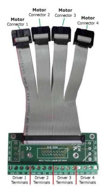
The Screw Terminal Adapter assists Mk1 and Mk2 controller connect to motor drivers that use screw terminal inputs. The adapter is compact. The ribbon cable connector helps in keeping enclosure wiring neat and accessible. Use is not difficult.
