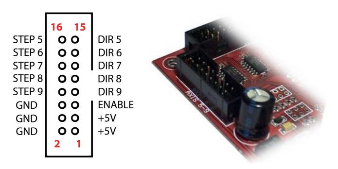
This connector controls up to 5 motor drivers. It can also provide an ENABLE signal to drivers that can take advantage of these feature.
