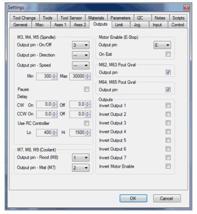
If you use 2 relays and 0-10V put jumper to "S" position set output pins like this:
