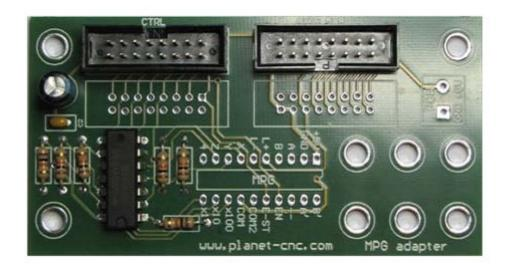
This adapter allows the Mk2 9-axis controller to support use of an MPG pendant, such as HEDSS pendant. This type of hand held device provides a convenient means of precise control while the operator is close by the machine. It can be of much assistance when performing job setup.
