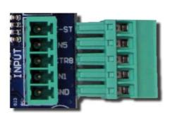
Four inputs are available on INPUT terminals.
