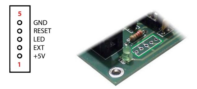
**GND:** Ground or 'common' connections.
