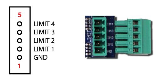
LIMIT 1-4 connects limit switches. It's recommended that a 100nF capacitor is connected directly across switch terminals.
