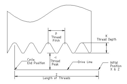
**Drive Line** - A line through the initial X position parallel to the Z.
