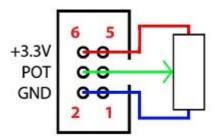
A potentiometer attached to this connector provides a manual jog speed control when using jogging keyboard connected to *JOG* connector.
