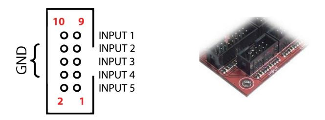
This connector will provide input for user-assigned functions.
