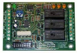
Output Board Adds Relays and VFD
