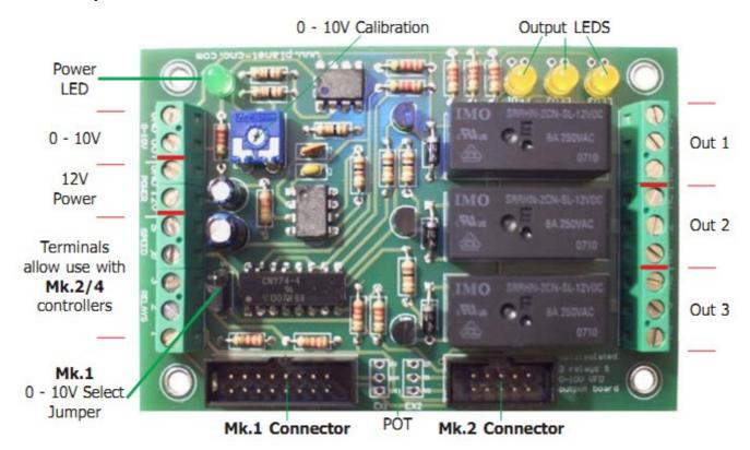
The output board assists controlled switching of external devices such as spindles, coolant pumps, dust extractors and so forth. It's a very easy way to add device switching. All planet-cnc.com controllers can use the output board. Screw terminal inputs allow this board to be used by almost any CNC controller.
