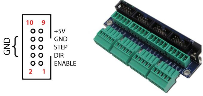
Each connector controls one motor driver.
