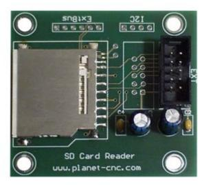
SD card options for the Mk2 CNC USB Controller are in development. Use of this adapter, in conjunction with control buttons attached to the INPUT connector, will allow CNC machinery to run proven NC programs without need of an attached PC.
