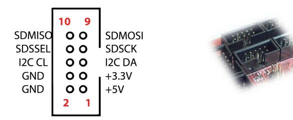
This connector allows use of SD Card and I2C protocol devices. An inexpensive I2C LCD digital readout has been successfully prototyped, tested and documented.
