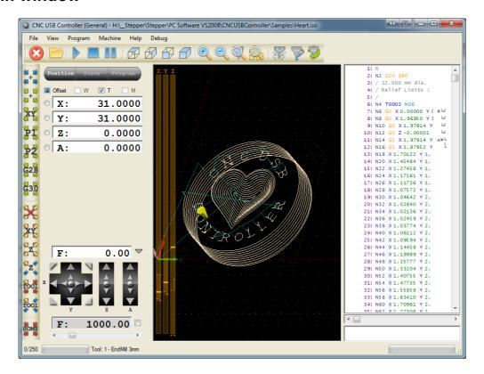
On launch of CNC USB Controller software the 'Main Window' will display. Data and status information for all aspects of G-Code program execution is provided on this main screen. The interface has been designed to be simple to use. Many regularly used functions are available via on-screen buttons and keyboard 'hot-keys'.
