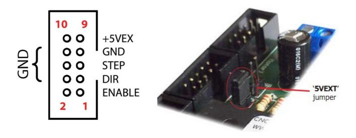
Each connector controls one motor driver.
