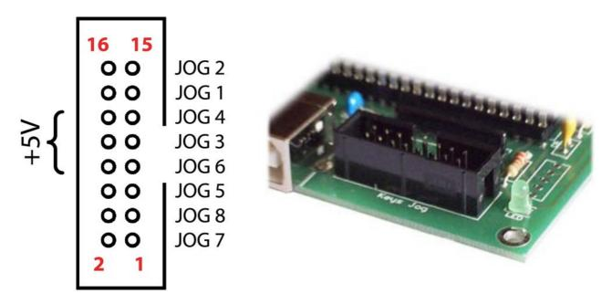
Manual jogging is controlled by switched operation of JOG 1-8. An optional plug-in 'Jogging Keyboard' can be provided. If users construct their own jogging keyboard, it's recommended that a 100nF capacitor is connected across switch terminals.
